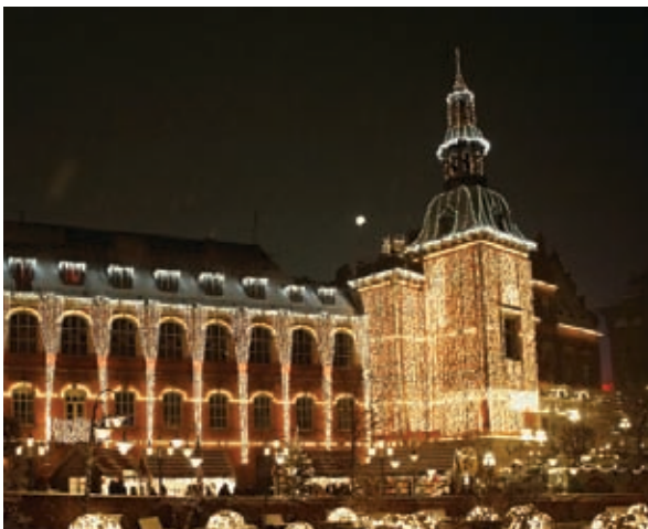
The new lighting on the Hans Christian Andersen Castle consisted of a mixture of decorative light chains with incandescent bulbs and LED hanging as long curtains which seemed to be tied with luminous, red bows.
